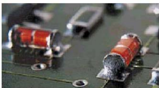
Cylindrical end cap terminations (MELF) (unit: mm)
