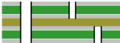
HDI PCB 4ML Laser drilled
