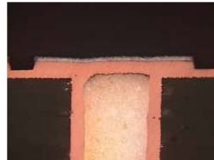
Cross section of plug vias
